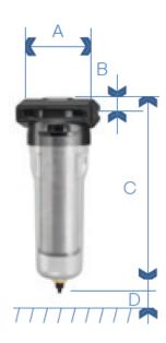
Dimensions filter housing (in inches – see factory for metric)
