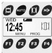
2. A WARNING
