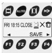
6. To **delete** a setting choose the desired setting by pressing F2(▼) and F3(▲) to scroll down and up.
