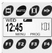
2. To **alter** a setting, choose the desired setting by pressing F2(▼) and F3(▲) to scroll down and up.
