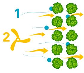
Nautilus filter technology uses filter media of a lower density than in classic coalescing filter technology.
