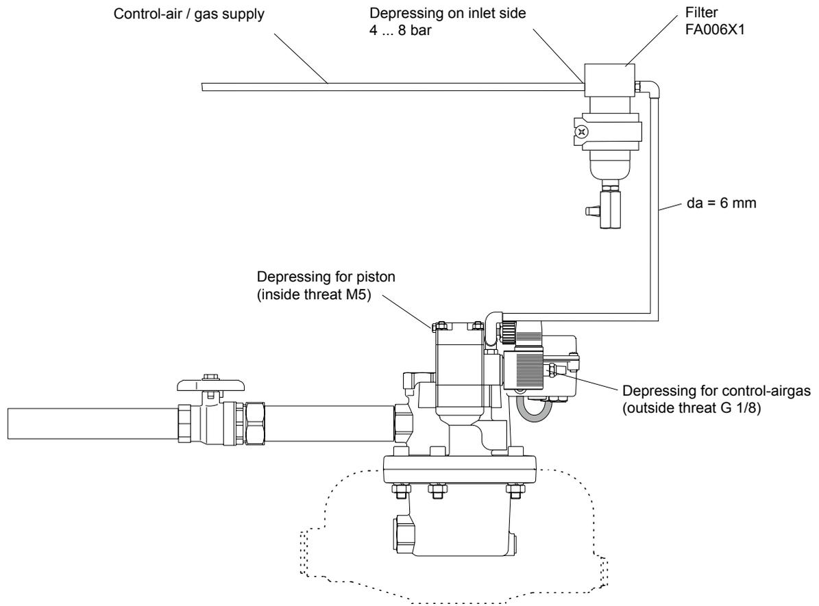
Installation BEKOMAT 3 E Ex 63 / 6 E Ex 25 at the control-air / gas depressing and depressing of piston
