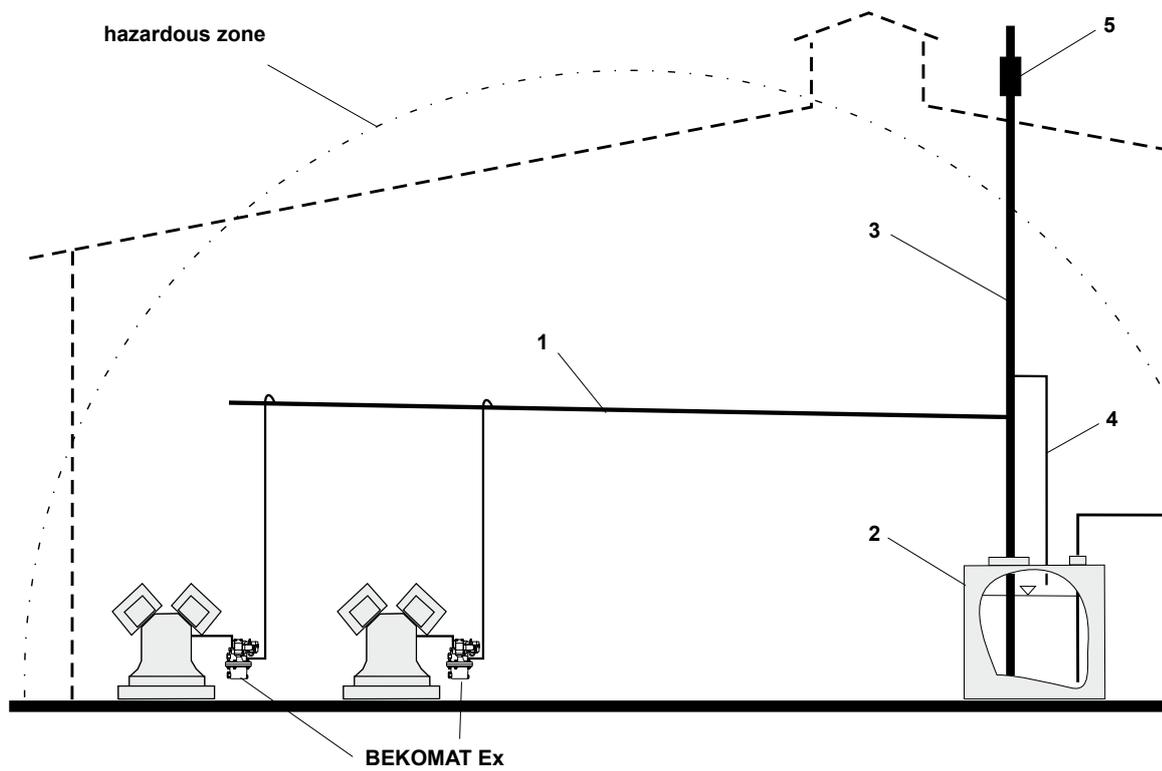
Compressor, condensate discharge and treatment in hazardous zones
