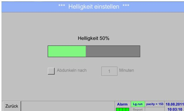
Here, the desired *brightness* (15 ... 100%) of the display can directly be set.
