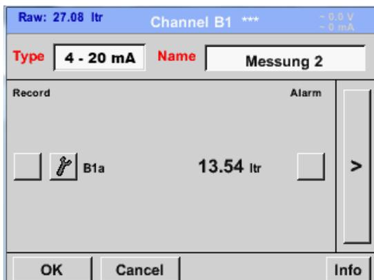
Scaling of the sensor (here, for example, *type 0 – 20 mA* - corresponds to 0 – 25 bar) can be found in the data sheet of the connected sensor.
