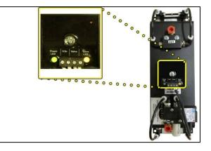
8.4.2 Use a Voltmeter to measure the voltage across the set of "Valve" terminals.
