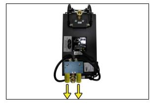
**8.2.5** Place your hand beneath the 4 way valve and feel for purging air.
