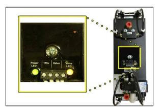
If either light is off see sections 8.3 and 8.4 to verify the cycle timer has correct voltages.
